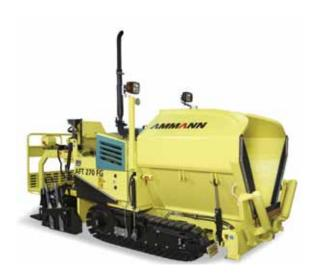
Tracked machine with rubber pads; automatic tensioning device system with grease accumulator. Hydrostatic transmission with two variable flow rate pumps which feed two motors with two displacements directly fastened to the planetary gearboxes which operate the tracks. Mounted on each pump, an electronic and proportional control gives a progressive start and stop, keeping the set speed constant. The steering-wheel is electronically controlled, the speed is constant when
