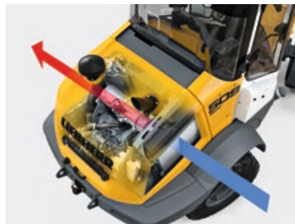
Cooling system L 507/L 509
